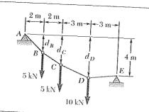
Determine (a) distance  $d_C$  for which portion DE of the cable is horizontal, (b) the corresponding reactions at A and E.
