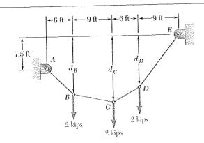
If  $d_C = 15$  ft, determine (a) the distances  $d_B$  and  $d_D$ , (b) the maximum tension in the cable.
