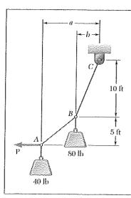
Cable ABC supports two loads as shown. Knowing that b = 4 ft, determine (a) the required magnitude of the horizontal force **P**, (b) the corresponding distance a.
