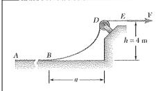
To the left of Point B the long cable ABDE rests on the rough horizontal surface shown. Knowing that the mass per unit length of the cable is 2 kg/m, determine the force F when a = 3.6 m.
