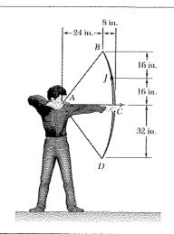
For the bow of Problem 7.9, determine the magnitude and location of the maximum (a) axial force, (b) shearing force, (c) bending moment.
