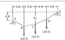
If  $d_C = 4.5$  ft, determine (a) the reaction at A, (b) the reaction at E.
