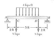
For the beam and loading shown, (a) draw the shear and bendingmoment diagrams, (b) determine the maximum absolute values of the shear and bending moment.
