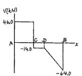
$|V|_{\text{max}} = 64.0 \text{ kN} \blacktriangleleft$
