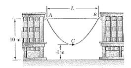
A 30-m cable is strung as shown between two buildings. The maximum tension is found to be 500 N, and the lowest point of the cable is observed to be 4 m above the ground. Determine (a) the horizontal distance between the buildings, (b) the total mass of the cable.
