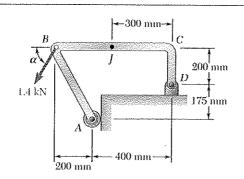
Determine the internal forces at Point J when  $\alpha = 90^{\circ}$ .
