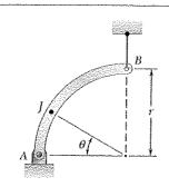
A quarter-circular rod of weight W and uniform cross section is supported as shown. Determine the bending moment at Point J when  $\theta = 30^{\circ}$ .
