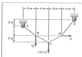
If a = 3 m, determine the magnitudes of **P** and **Q** required to maintain the cable in the shape shown.
