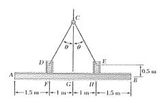
For the structural member of Problem 7.50, determine (a) the angle  $\theta$  for which the maximum absolute value of the bending moment in beam AB is as small as possible, (b) the corresponding value of  $|M|_{\text{max}}$ . (Hint: Draw the bending-moment diagram and then equate the absolute values of the largest positive and negative bending moments obtained.)
