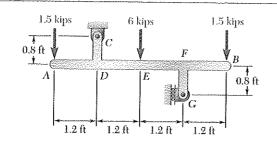
Draw the shear and bending-moment diagrams for the beam AB, and determine the maximum absolute values of the shear and bending moment.
