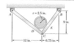
A 5-in.-diameter pipe is supported every 9 ft by a small frame consisting of two members as shown. Knowing that the combined weight of the pipe and its contents is 10 lb/ft and neglecting the effect of friction, determine the magnitude and location of the maximum bending moment in member AC.
