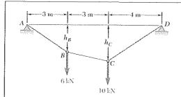
Two loads are suspended as shown from the cable *ABCD*. Knowing that  $h_B = 1.8$  m, determine (a) the distance  $h_C$ , (b) the components of the reaction at D, (c) the maximum tension in the cable.
