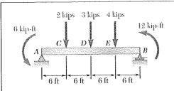
For the beam and loading shown, (a) draw the shear and bending-moment diagrams, (b) determine the maximum absolute values of the shear and bending moment.
