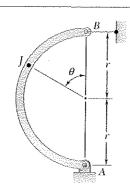
A semicircular rod of weight W and uniform cross section is supported as shown. Determine the bending moment at Point J when  $\theta = 60^{\circ}$ .
