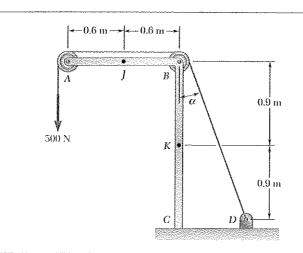
Knowing that the radius of each pulley is 150 mm, that  $\alpha = 30^{\circ}$ , and neglecting friction, determine the internal forces at (a) Point J, (b) Point K.
