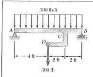
(a) Draw the shear and bending-moment diagrams for beam AB, (b) determine the magnitude and location of the maximum absolute value of the bending moment.
