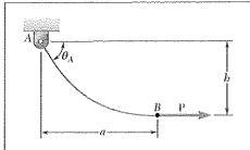
A uniform cable weighing 3 lb/ft is held in the position shown by a horizontal force **P** applied at *B*. Knowing that P = 180 lb and  $\theta_A = 60^{\circ}$ , determine (a) the location of Point *B*, (b) the length of the cable.
