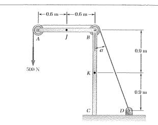
Knowing that the radius of each pulley is 150 mm, that  $\alpha = 20^{\circ}$ , and neglecting friction, determine the internal forces at (a) Point J, (b) Point K.
