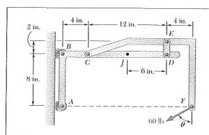
Determine the internal forces (axial force, shearing force, and bending moment) at Point J of the structure indicated.
