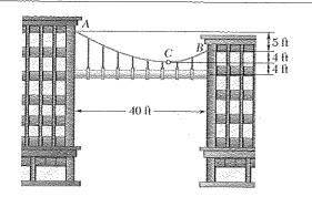
A steam pipe weighting 45 lb/ft that passes between two buildings 40 ft apart is supported by a system of cables as shown. Assuming that the weight of the cable system is equivalent to a uniformly distributed loading of 5 lb/ft, determine (a) the location of the lowest Point C of the cable, (b) the maximum tension in the cable.
