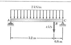
For the beam and loading shown, (a) draw the shear and bending-moment diagrams, (b) determine the maximum absolute values of the shear and bending moment.
