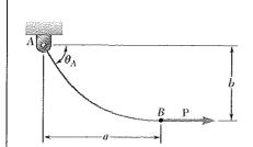
A uniform cable weighing 3 lb/ft is held in the position shown by a horizontal force **P** applied at *B*. Knowing that P = 150 lb and  $\theta_A = 60^\circ$ , determine (a) the location of Point *B*, (b) the length of the cable.
