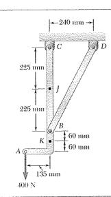
Determine the internal forces at Point K of the structure shown.
