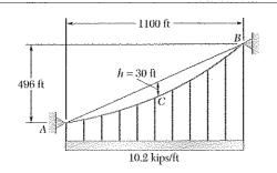
Each cable of the side spans of the Golden Gate Bridge supports a load w = 10.2 kips/ft along the horizontal. Knowing that for the side spans the maximum vertical distance h from each cable to the chord AB is 30 ft and occurs at midspan, determine (a) the maximum tension in each cable, (b) the slope at B.
