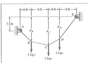
Determine (a) the distance  $d_C$  for which portion BC of the cable is horizontal, (b) the corresponding components of the reaction at E.
