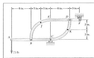
Two members, each consisting of a straight and a quarter-circular portion of rod, are connected as shown and support a 75-lb load at A. Determine the internal forces at Point K.
