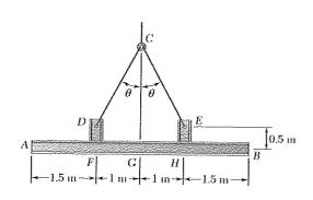
Two small channel sections DF and EH have been welded to the uniform beam AB of weight W=3 kN to form the rigid structural member shown. This member is being lifted by two cables attached at D and E. Knowing that  $\theta=30^{\circ}$  and neglecting the weight of the channel sections, (a) draw the shear and bending-moment diagrams for beam AB, (b) determine the maximum absolute values of the shear and bending moment in the beam.
