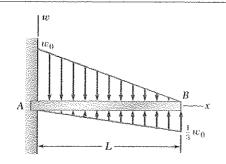
For the beam and loading shown, (a) write the equations of the shear and bending-moment curves, (b) determine the magnitude and location of the maximum bending moment.
