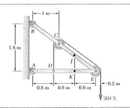
Knowing that the radius of each pulley is 200 mm and neglecting friction, determine the internal forces at Point Jof the frame shown.
