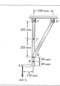
Determine the internal forces at Point J of the structure shown.
