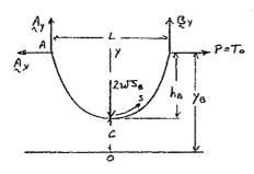
$$s_T = 20 \text{ m} \rightarrow s_B = \frac{20 \text{ m}}{2} = 10 \text{ m}$$
