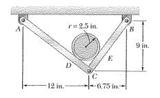
For the frame of Problem 7.19, determine the magnitude and location of the maximum bending moment in member BC.
