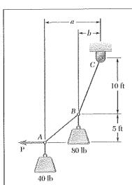
Cable ABC supports two loads as shown. Determine the distances a and b when a horizontal force **P** of magnitude 60 lb is applied at A.
