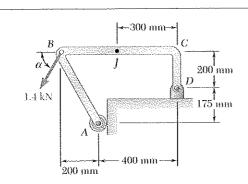
Determine the internal forces at Point J when  $\alpha = 0$ .
