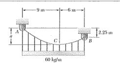
Cable ACB supports a load uniformly distributed along the horizontal as shown. The lowest Point C is located 9 m to the right of A. Determine (a) the vertical distance a, (b) the length of the cable, (c) the components of the reaction at A.
