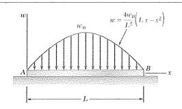
The beam AB, which lies on the ground, supports the parabolic load shown. Assuming the upward reaction of the ground to be uniformly distributed, (a) write the equations of the shear and bending-moment curves, (b) determine the maximum bending moment.
