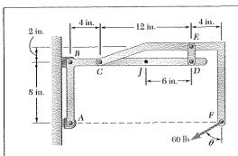
Determine the internal forces (axial force, shearing force, and bending moment) at Point J of the structure indicated.
