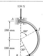
A semicircular rod is loaded as shown. Determine the internal forces at Point J.
