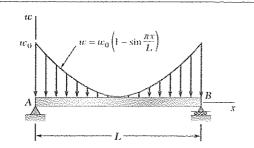
For the beam and loading shown, (a) write the equations of the shear and bending-moment curves, (b) determine the maximum bending moment.
