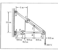
Knowing that the radius of each pulley is 200 mm and neglecting friction, determine the internal forces at Point *J* of the frame shown.
