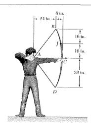
An archer aiming at a target is pulling with a 45-lb force on the bowstring. Assuming that the shape of the bow can be approximated by a parabola, determine the internal forces at Point J.
