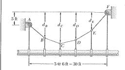
An oil pipeline is supported at 6-ft intervals by vertical hangers attached to the cable shown. Due to the combined weight of the pipe and its contents the tension in each hanger is 400 lb. Knowing that  $d_C = 12$  ft, determine (a) the maximum tension in the cable, (b) the distance  $d_D$ .
