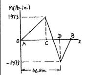
$$M_{\text{max}} = |M_{\text{min}}| \text{ or } M_C = -M_D: 13,500 \left(1 - \frac{40}{a}\right) = 150(60 - a)$$
