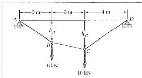
Knowing that the maximum tension in cable ABCD is 15 kN, determine (a) the distance  $h_R$ , (b) the distance  $h_C$ .
