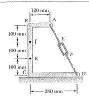
It has been experimentally determined that the bending moment at Point K of the frame shown is 300 N · m. Determine (a) the tension in rods AE and FD, (b) the corresponding internal forces at Point J.
