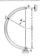
A semicircular rod of weight W and uniform cross section is supported as shown. Determine the bending moment at Point J when  $\theta = 150^{\circ}$ .
