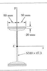
Two 20-mm steel plates are welded to a rolled S section as shown. Determine the moments of inertia and the radii of gyration of the combined section with respect to the centroidal x and y axes.
