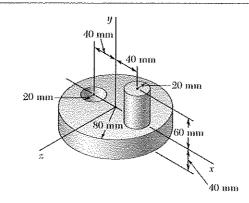
The machine element shown is fabricated from steel. Determine the mass moment of inertia of the assembly with respect to (a) the x axis, (b) the y axis, (c) the z axis. (The density of steel is  $7850 \text{ kg/m}^3$ .)
