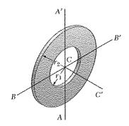
Determine the mass moment of inertia of a ring of mass m, cut from a thin uniform plate, with respect to (a) the axis AA', (b) the centroidal axis CC' that is perpendicular to the plane of the ring.
