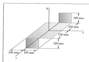
A 2-mm thick piece of sheet steel is cut and bent into the machine component shown. Knowing that the density of steel is 7850 kg/m³, determine the mass moment of inertia of the component with respect to each of the coordinate axes.
