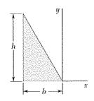
Determine by direct integration the product of inertia of the given area with respect to the x and y axes.
