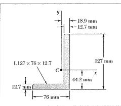
Determine the moments of inertia and the product of inertia of the L127×76×12.7-mm angle cross section of Problem 9.78 with respect to new centroidal axes obtained by rotating the x and y axes 45° counterclockwise.
