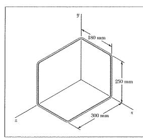
The figure shown is formed of 1.5-mm-diameter aluminum wire. Knowing that the density of aluminum is 2800 kg/m<sup>3</sup>, determine the mass products of inertia  $I_{xy}$ ,  $I_{yz}$ , and  $I_{zx}$  of the wire figure.
