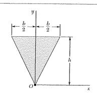
Determine the polar moment of inertia and the polar radius of gyration of the isosceles triangle shown with respect to Point O.
