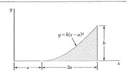
Determine by direct integration the moment of inertia of the shaded area with respect to the y axis.
