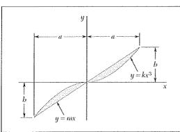
Determine the moment of inertia and the radius of gyration of the shaded area shown with respect to the y axis.
