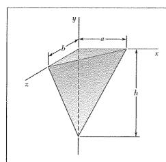
Determine by direct integration the mass moment of inertia with respect to the y axis of the tetrahedron shown, assuming that it has a uniform density and a mass m.
