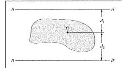
Determine for the shaded region the area and the moment of inertia with respect to the centroidal axis parallel to BB', knowing that  $d_1 = 25$  mm and  $d_2 = 15$  mm and that the moments of inertia with respect to AA' and BB' are  $7.84 \times 10^6$  mm<sup>4</sup> and  $5.20 \times 10^6$  mm<sup>4</sup>, respectively.
