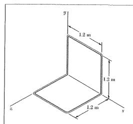
For the wire figure of Problem 9.148, determine the mass moment of inertia of the figure with respect to the axis through the origin characterized by the unit vector  $\lambda = (-3\mathbf{i} - 6\mathbf{j} + 2\mathbf{k})/7$ .
