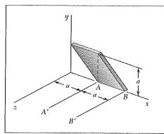
A thin plate of mass m was cut in the shape of a parallelogram as shown. Determine the mass moment of inertia of the plate with respect to (a) the y axis, (b) the axis AA', which is perpendicular to the plate.
