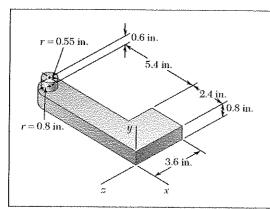
Determine the mass products of inertia  $I_{xy}$ ,  $I_{yz}$ , and  $I_{zx}$  of the cast aluminum machine component shown. (The specific weight of aluminum is  $0.100 \text{ lb/in.}^3$ )
