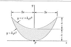
Determine the polar moment of inertia and the polar radius of gyration of the shaded area shown with respect to Point P.
