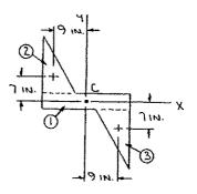
where, using the results of Sample Problem 9.6,  $\overline{I}_{x'y'} = -\frac{1}{72}b^2h^2$  for both triangles. Note that the sign of  $\overline{I}_{x'y'}$  is unchanged because the angles of rotation are  $0^{\circ}$  and  $180^{\circ}$  for triangles 2 and 3, respectively.
