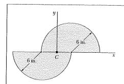
Using the parallel-axis theorem, determine the product of inertia of the area shown with respect to the centroidal x and y axes.
