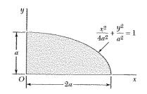
Using Mohr's circle, determine for the quarter ellipse of Problem 9.67 the moments of inertia and the product of inertia with respect to new axes obtained by rotating the x and y axes about O(a) through  $45^{\circ}$  counterclockwise, (b) through  $30^{\circ}$  clockwise.
