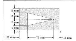
Determine the moments of inertia  $\overline{I}_x$  and  $\overline{I}_y$  of the area shown with respect to centroidal axes respectively parallel and perpendicular to side AB.
