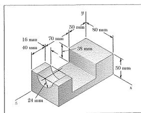
Determine the mass moment of inertia of the steel fixture of Problems 9.145 and 9.149 with respect to the axis through the origin that forms equal angles with the x, y, and z axes.
