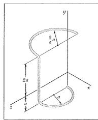
Brass wire with a weight per unit length w is used to form the figure shown. Determine the mass products of inertia  $I_{xy}$ ,  $I_{yz}$ , and  $I_{zx}$  of the wire figure.
