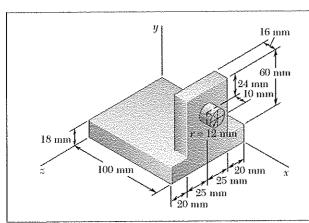
Determine the mass products of inertia  $I_{xy}$ ,  $I_{yz}$ , and  $I_{zx}$  of the steel machine element shown. (The density of steel is  $7850 \text{ kg/m}^3$ .)
