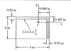
Determine the moments of inertia and the product of inertia of the  $L3\times2\times\frac{1}{4}$ -in. angle cross section of Problem 9.74 with respect to new centroidal axes obtained by rotating the x and y axes 30° clockwise.
