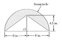
Determine the polar moment of inertia of the area shown with respect to (a) Point O, (b) the centroid of the area.
