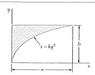
Determine by direct integration the product of inertia of the given area with respect to the x and y axes.
