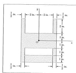
Determine the moment of inertia and the radius of gyration of the shaded area with respect to the *x* axis.
