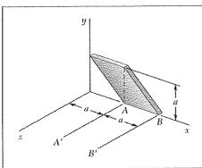
A thin plate of mass m was cut in the shape of a parallelogram as shown. Determine the mass moment of inertia of the plate with respect to (a) the x axis, (b) the axis BB', which is perpendicular to the plate.
