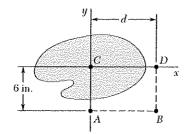
The shaded area is equal to 50 in.<sup>2</sup>. Determine its centroidal moments of inertia  $\overline{I}_x$  and  $\overline{I}_y$ , knowing that  $\overline{I}_y = 2\overline{I}_x$  and that the polar moment of inertia of the area about Point A is  $J_A = 2250$  in.<sup>4</sup>.
