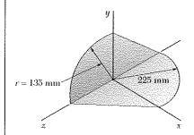
A section of sheet steel 2 mm thick is cut and bent into the machine component shown. Knowing that the density of steel is 7850 kg/m<sup>3</sup>, determine the mass products of inertia  $I_{xy}$ ,  $I_{yz}$ , and  $I_{zx}$  of the component.
