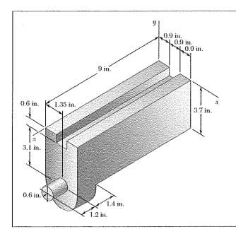
Determine the mass moment of inertia of the steel machine element shown with respect to the y axis. (The specific weight of steel is 490 lb/ft<sup>3</sup>.)
