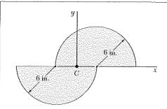
Determine the moments of inertia and the product of inertia of the area of Problem 9.73 with respect to new centroidal axes obtained by rotating the x and y axes  $60^{\circ}$  counterclockwise.
