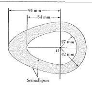
Determine the polar moment of inertia of the area shown with respect to (a) Point O, (b) the centroid of the area.
