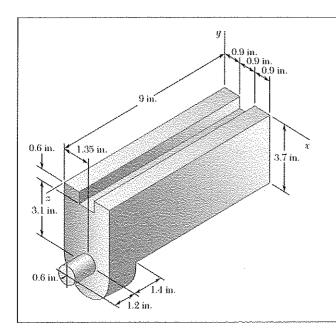
Determine the mass moment of inertia of the steel machine element shown with respect to the z axis. (The specific weight of steel is 490 lb/ft<sup>3</sup>.)
