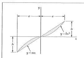
Determine the moment of inertia and the radius of gyration of the shaded area shown with respect to the x axis.
