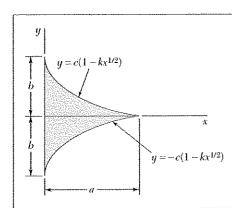
Determine by direct integration the moment of inertia of the shaded area with respect to the y axis.
