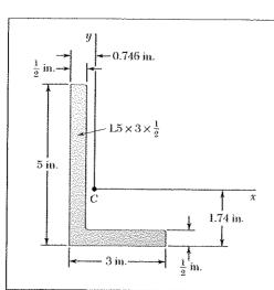
Using the parallel-axis theorem, determine the product of inertia of the L5  $\times$  3  $\times$   $\frac{1}{2}$ -in. angle cross section shown with respect to the centroidal x and y axes.
