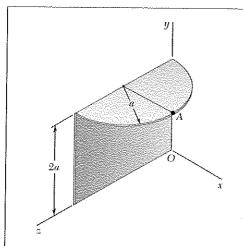
A piece of sheet steel of thickness t and specific weight  $\gamma$  is cut and bent into the machine component shown. Determine the mass moment of inertia of the component with respect to the joining the origin O and Point A.
