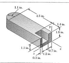
Determine the mass products of inertia  $I_{xy}$ ,  $I_{yz}$ , and  $I_{zx}$  of the cast aluminum machine component shown. (The specific weight of aluminum is  $0.100 \text{ lb/in.}^3$ )
