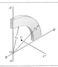
The quarter ring shown has a mass m and was cut from a thin, uniform plate. Knowing that  $r_1 = \frac{3}{4} r_2$ , determine the mass moment of inertia of the quarter ring with respect to (a) the axis AA', (b) the centroidal axis CC' that is perpendicular to the plane of the quarter ring.
