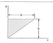
Determine by direct integration the moment of inertia of the shaded area with respect to the y axis.
