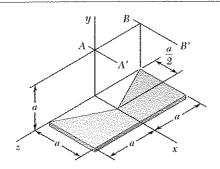
A piece of thin, uniform sheet metal is cut to form the machine component shown. Denoting the mass of the component by m, determine its mass moment of inertia with respect to (a) the x axis, (b) the y axis.
