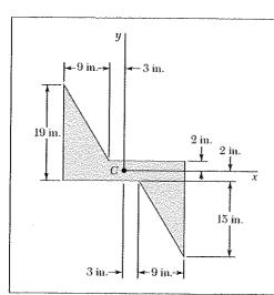
Using Mohr's circle, determine for the area indicated the orientation of the principal centroidal axes and the corresponding values of the moments of inertia.
