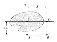
The polar moments of inertia of the shaded area with respect to Points A, B, and D are, respectively,  $J_A = 2880$  in.<sup>4</sup>,  $J_B = 6720$  in.<sup>4</sup>, and  $J_D = 4560$  in.<sup>4</sup>. Determine the shaded area, its centroidal moment of inertia  $\overline{J}_C$ , and the distance d from C to D.
