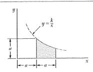
Determine by direct integration the moment of inertia of the shaded area with respect to the x axis.
