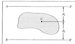
For the 4000-mm<sup>2</sup> shaded area shown, determine the distance  $d_2$  and the moment of inertia with respect to the centroidal axis parallel to AA' knowing that the moments of inertia with respect to AA' and BB' are  $12\times10^6$  mm<sup>4</sup> and  $23.9\times10^6$  mm<sup>4</sup>, respectively, and that  $d_1 = 25$  mm.
