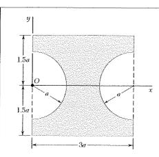
Determine the moments of inertia of the shaded area shown with respect to the x and y axes when a = 20 mm.
