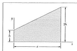
The area shown is revolved about the x axis to form a homogeneous solid of revolution of mass m. Using direct integration, express the mass moment of inertia of the solid with respect to the x axis in terms of m and h.
