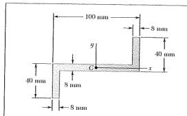
Using Mohr's circle, determine the moments of inertia and the product of inertia of the area of Problem 9.75 with respect to new centroidal axes obtained by rotating the x and y axes 45° clockwise.
