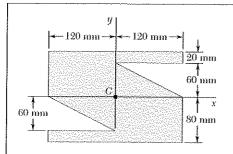
Using Mohr's circle, determine the moments of inertia and the product of inertia of the area of Problem 9.72 with respect to new centroidal axes obtained by rotating the x and y axes  $30^{\circ}$  counterclockwise.
