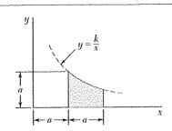
Determine by direct integration the moment of inertia of the shaded area with respect to the y axis.
