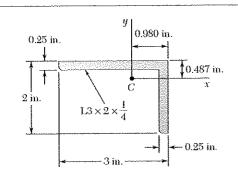
Using the parallel-axis theorem, determine the product of inertia of the area shown with respect to the centroidal x and y axes.
