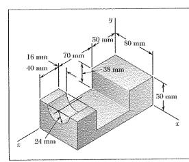
Determine the mass products of inertia  $I_{xy}$ ,  $I_{yz}$ , and  $I_{zx}$  of the steel fixture shown. (The density of steel is 7850 kg/m<sup>3</sup>.)
