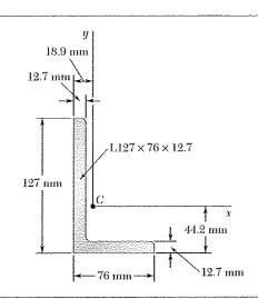
Using Mohr's circle, determine for the cross section of the rolledsteel angle shown the orientation of the principal centroidal axes and the corresponding values of the moments of inertia. (Properties of the cross sections are given in Figure 9.13.)
