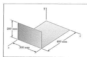
A section of sheet steel 2 mm thick is cut and bent into the machine component shown. Knowing that the density of steel is 7850 kg/m<sup>3</sup>, determine the mass products of inertia  $I_{xy}$ ,  $I_{yz}$ , and  $I_{zx}$  of the component.
