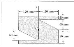
Using the parallel-axis theorem, determine the product of inertia of the area shown with respect to the centroidal x and y axes.
