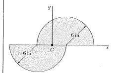
Using Mohr's circle, determine the moments of inertia and the product of inertia of the area of Problem 9.73 with respect to new centroidal axes obtained by rotating the x and y axes  $60^{\circ}$  counterclockwise.
