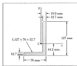
For the angle cross section indicated, determine the orientation of the principal axes at the origin and the corresponding values of the moments of inertia.
