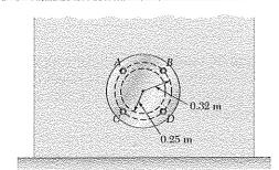
The cover for a 0.5-m-diameter access hole in a water storage tank is attached to the tank with four equally spaced bolts as shown. Determine the additional force on each bolt due to the water pressure when the center of the cover is located 1.4 m below the water surface.
