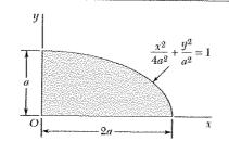
For the quarter ellipse of Problem 9.67, use Mohr's circle to determine the orientation the principal axes at the origin and the corresponding values of the moments of inertia.
