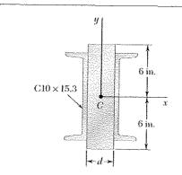
Two channels are welded to a  $d \times 12$ -in. steel plate as shown. Determine the width d for which the ratio  $\overline{I_x}/\overline{I_y}$  of the centroidal moments of inertia of the section is 16.
