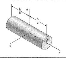
Determine by direct integration the mass moment of inertia with respect to the y axis of the right circular cylinder shown, assuming that it has a uniform density and a mass m.
