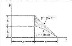
Determine the moment of inertia and the radius of gyration of the shaded area shown with respect to the y axis.
