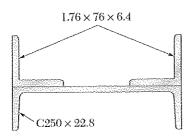
Two L76  $\times$  76  $\times$  6.4-mm angles are welded to a C250  $\times$  22.8 channel. Determine the moments of inertia of the combined section with respect to centroidal axes respectively parallel and perpendicular to the web of the channel.
