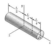
For the homogeneous circular cylinder shown, of radius a and length L, determine the value of the ratio a/L for which the ellipsoid of inertia of the cylinder is a sphere when computed (a) at the centroid of the cylinder, (b) at Point A.
