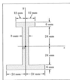
Determine the moment of inertia and the radius of gyration of the shaded area with respect to the x axis.
