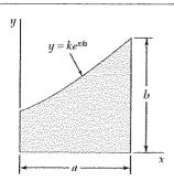
Determine by direct integration the moment of inertia of the shaded area with respect to the y axis.
