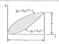
Determine the moment of inertia and the radius of gyration of the shaded area shown with respect to the x axis.
