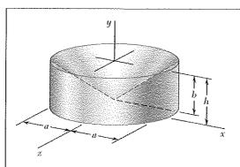
The machine part shown is formed by machining a conical surface into a circular cylinder. For  $b = \frac{1}{2}h$ , determine the mass moment of inertia and the radius of gyration of the machine part with respect to the y axis.
