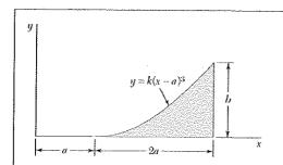
Determine by direct integration the moment of inertia of the shaded area with respect to the x axis.
