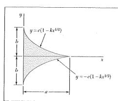
Determine by direct integration the moment of inertia of the shaded area with respect to the x axis.
