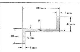
Determine the moments of inertia and the product of inertia of the area of Problem 9.75 with respect to new centroidal axes obtained by rotating the x and y axes 45° clockwise.
