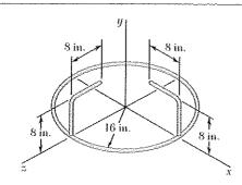
For the wire figure of Problem 9.46, determine the mass moment of inertia of the figure with respect to the axis through the origin characterized by the unit vector  $\lambda = (-3\mathbf{i} - 6\mathbf{j} + 2\mathbf{k})/7$ .
