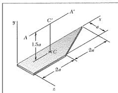
A thin plate of mass m has the trapezoidal shape shown. Determine the mass moment of inertia of the plate with respect to (a) the x axis, (b) the y axis.
