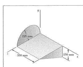
Determine the mass moment of inertia of the machine component of Problems 9.136 and 9.155 with respect to the axis through the origin characterized by the unit vector  $\lambda = (-4\mathbf{i} + 8\mathbf{j} + \mathbf{k})/9$ .
