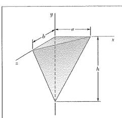
Determine by direct integration the mass moment of inertia with respect to the x axis of the tetrahedron shown, assuming that it has a uniform density and a mass m.
