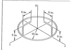
Aluminum wire with a weight per unit length of 0.033 lb/ft is used to form the circle and the straight members of the figure shown. Determine the mass moment of inertia of the assembly with respect to each of the coordinate axes.
