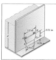
A vertical trapezoidal gate that is used as an automatic valve is held shut by two springs attached to hinges located along edge AB. Knowing that each spring exerts a couple of magnitude 1470 N·m, determine the depth d of water for which the gate will open.
