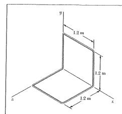
A homogeneous wire with a mass per unit length of 0.056 kg/m is used to form the figure shown. Determine the mass moment of inertia of the wire with respect to each of the coordinate axes.
