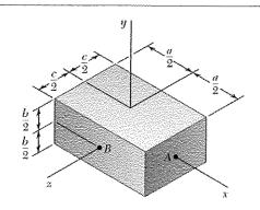
For the rectangular prism shown, determine the values of the ratios b/a and c/a so that the ellipsoid of inertia of the prism is a sphere when computed (a) at Point A, (b) at Point B.
