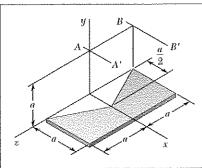
A piece of thin, uniform sheet metal is cut to form the machine component shown. Denoting the mass of the component by m, determine its mass moment of inertia with respect to (a) the axis AA', (b) the axis BB', where the AA' and BB' axes are parallel to the x axis and lie in a plane parallel to and at a distance a above the xz plane.
