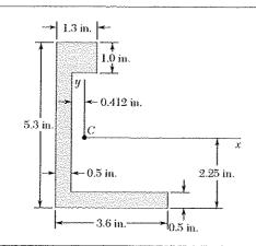
Using Mohr's circle, determine for the area indicated the orientation of the principal centroidal axes and the corresponding values of the moments of inertia.
