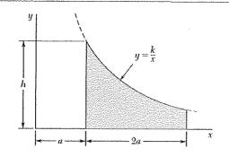
The area shown is revolved about the x axis to form a homogeneous solid of revolution of mass m. Determine by direct integration the mass moment of inertia of the solid with respect to (a) the x axis, (b) the y axis. Express your answers in terms of m and the dimensions of the solid.
