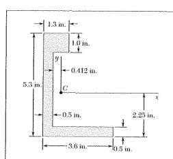
Using the parallel-axis theorem, determine the product of inertia of the area shown with respect to the centroidal x and y axes.
