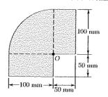
Determine the polar moment of inertia of the area shown with respect to (a) Point O, (b) the centroid of the area.
