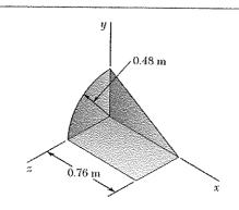
A 2-mm thick piece of sheet steel is cut and bent into the machine component shown. Knowing that the density of steel is 7850 kg/m³, determine the mass moment of inertia of the component with respect to each of the coordinate axes.
