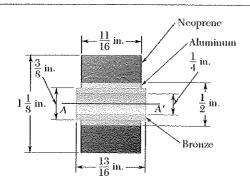
Shown is the cross section of an idler roller. Determine its mass moment of inertia and its radius of gyration with respect to the axis AA'. (The specific weight of bronze is  $0.310 \text{ lb/in}^3$ ; of aluminum,  $0.100 \text{ lb/in}^3$ ; and of neoprene,  $0.0452 \text{ lb/in}^3$ .)
