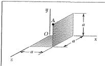
The thin bent plate shown is of uniform density and weight W. Determine its mass moment of inertia with respect to the line joining the origin O and Point A.
