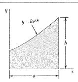
Determine by direct integration the moment of inertia of the shaded area with respect to the x axis.
