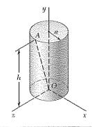
The homogeneous circular cylinder shown has a mass m. Determine the mass moment of inertia of the cylinder with respect to the line joining the origin O and Point A that is located on the perimeter of the top surface of the cylinder.
