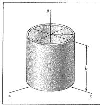
Knowing that the thin cylindrical shell shown is of mass m, thickness t, and height h, determine the mass moment of inertia of the shell with respect to the x axis. (*Hint*: Consider the shell as formed by removing a cylinder of radius a and height h from a cylinder of radius a + t and height h; then neglect terms containing  $t^2$  and  $t^3$  and keep those terms containing t.)
