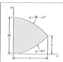
Determine the moment of inertia and the radius of gyration of the shaded area shown with respect to the y axis.
