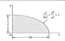
Determine by direct integration the product of inertia of the given area with respect to the x and y axes.
