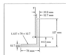
Using the parallel-axis theorem, determine the product of inertia of the area shown with respect to the centroidal x and y axes.
