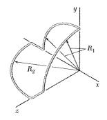
Thin aluminum wire of uniform diameter is used to form the figure shown. Denoting by m' the mass per unit length of the wire, determine the mass products of inertia  $I_{xy}$ ,  $I_{yz}$ , and  $I_{zx}$  of the wire figure.
