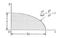
For the quarter ellipse of Problem 9.67, determine the orientation of the principal axes at the origin and the corresponding values of the moments of inertia.
