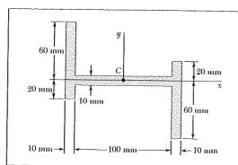
Using the parallel-axis theorem, determine the product of inertia of the area shown with respect to the centroidal x and y axes.
