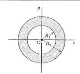
(a) Show that the polar radius of gyration  $k_O$  of the annular area shown is approximately equal to the mean radius  $R_m = (R_1 + R_2)/2$  for small values of the thickness  $t = R_2 - R_1$ . (b) Determine the percentage error introduced by using  $R_m$  in place of  $k_O$  for the following values of  $t/R_m$ :  $1, \frac{1}{2}$ , and  $\frac{1}{10}$ .
