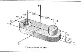
Determine the mass moments of inertia and the radii of gyration of the steel machine element shown with respect to the x and y axes. (The density of steel is  $7850 \text{ kg/m}^3$ .)
