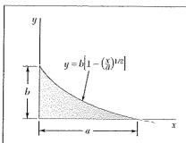
Determine the moments of inertia and the radii of gyration of the shaded area shown with respect to the x and y axes.
