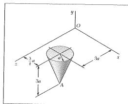
The homogeneous circular cone shown has a mass m. Determine the mass moment of inertia of the cone with respect to the line joining the origin O and Point A.
