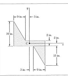
Using the parallel-axis theorem, determine the product of inertia of the area shown with respect to the centroidal x and y axes.
