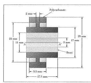
Shown is the cross section of a molded flat-belt pulley. Determine its mass moment of inertia and its radius of gyration with respect to the axis AA'. (The density of brass is  $8650 \text{ kg/m}^3$  and the density of the fiber-reinforced polycarbonate used is  $1250 \text{ kg/m}^3$ .)
