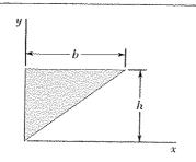
Determine by direct integration the moment of inertia of the shaded area with respect to the x axis.
