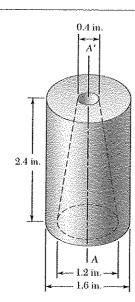
Determine the mass moment of inertia of the 0.9-lb machine component shown with respect to the axis AA'.
