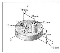
For the component described in Problem 9.165, determine (a) the principal mass moments of inertia at the origin, (b) the principal axes of inertia at the origin. Sketch the body and show the orientation of the principal axes of inertia relative to the x, y, and z axes.
