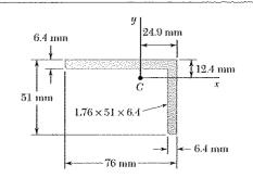
Using Mohr's circle, determine for the cross section of the rolledsteel angle shown the orientation of the principal centroidal axes and the corresponding values of the moments of inertia. (Properties of the cross sections are given in Figure 9.13.)
