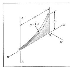
The parabolic spandrel shown was cut from a thin, uniform plate. Denoting the mass of the spandrel by m, determine its mass moment of inertia with respect to (a) the axis BB', (b) the axis DD' that is perpendicular to the spandrel. (*Hint:* See Sample Problem 9.3.)
