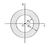
(a) Determine by direct integration the polar moment of inertia of the annular area shown with respect to Point O. (b) Using the result of Part a, determine the moment of inertia of the given area with respect to the x axis.
