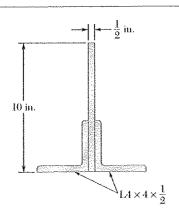
Two L4  $\times$  4  $\times$   $\frac{1}{2}$ -in. angles are welded to a steel plate as shown. Determine the moments of inertia of the combined section with respect to centroidal axes respectively parallel and perpendicular to the plate.
