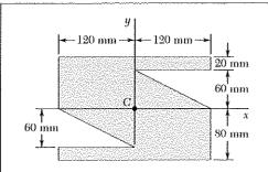
For the area indicated, determine the orientation of the principal axes at the origin and the corresponding values of the moments of inertia.
