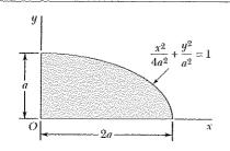
Determine for the quarter ellipse of Problem 9.67 the moments of inertia and the product of inertia with respect to new axes obtained by rotating the x and y axes about O(a) through  $45^{\circ}$  counterclockwise, (b) through  $30^{\circ}$  clockwise.
