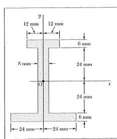
Determine the moment of inertia and the radius of gyration of the shaded area with respect to the *y* axis.
