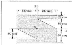
Determine the moments of inertia and the product of inertia of the area of Problem 9.72 with respect to new centroidal axes obtained by rotating the x and y axes 30° counterclockwise.
