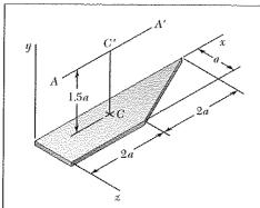
A thin plate of mass m has the trapezoidal shape shown. Determine the mass moment of inertia of the plate with respect to (a) the centroidal axis CC' that is perpendicular to the plate, (b) the axis AA' that is parallel to the x axis and is located at a distance 1.5a from the plate.
