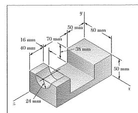
Determine the mass moment of inertia of the steel fixture shown with respect to (a) the x axis, (b) the y axis, (c) the z axis. (The density of steel is  $7850 \text{ kg/m}^3$ .)
