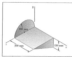
A 2-mm thick piece of sheet steel is cut and bent into the machine component shown. Knowing that the density of steel is 7850 kg/m³, determine the mass moment of inertia of the component with respect to each of the coordinate axes.
