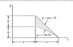
Determine the moment of inertia and the radius of gyration of the shaded area shown with respect to the x axis.
