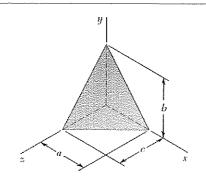
For the homogeneous tetrahedron of mass m shown, (a) determine by direct integration the mass product of inertia  $I_{zx}$ , (b) deduce  $I_{yz}$  and  $I_{xy}$  from the result obtained in Part a.
