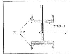
Two channels are welded to a rolled W section as shown. Determine the moments of inertia and the radii of gyration of the combined section with respect to the centroidal x and y axes.
