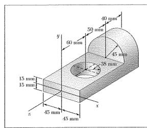
Determine the mass moment of inertia and the radius of gyration of the steel machine element shown with respect to the x axis. (The density of steel is  $7850 \text{ kg/m}^3$ .)
