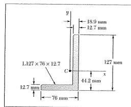
Using Mohr's circle, determine the moments of inertia and the product of inertia of the  $L127 \times 76 \times 12.7$ -mm angle cross section of Problem 9.78 with respect to new centroidal axes obtained by rotating the x and y axes 45° counterclockwise.
