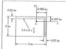
Using Mohr's circle, determine the moments of inertia and the product of inertia of the  $L3\times2\times\frac{1}{4}$ -in. angle cross section of Problem 9.74 with respect to new centroidal axes obtained by rotating the x and y axes 30° clockwise.
