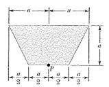
Determine the polar moment of inertia and the polar radius of gyration of the shaded area shown with respect to Point P.
