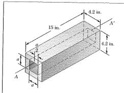
A square hole is centered in and extends through the aluminum machine component shown. Determine (a) the value of a for which the mass moment of inertia of the component with respect to the axis AA', which bisects the top surface of the hole, is maximum, (b) the corresponding values of the mass moment of inertia and the radius of gyration with respect to the axis AA'. (The specific weight of aluminum is  $0.100 \text{ lb/in.}^3$ .)
