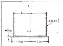
Two L5  $\times$  3  $\times$   $\frac{1}{2}$ -in. angles are welded to a  $\frac{1}{2}$ -in. steel plate. Determine the distance b and the centroidal moments of inertia  $\overline{I}_x$ and  $\overline{I}_y$  of the combined section, knowing that  $\overline{I}_y = 4\overline{I}_x$ .
