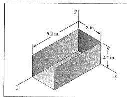
The cover for an electronic device is formed from sheet aluminum that is 0.05 in. thick. Determine the mass moment of inertia of the cover with respect to each of the coordinate axes. (The specific weight of aluminum is 0.100 lb/in.<sup>3</sup>.)
