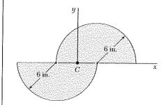
Using Mohr's circle, determine for the area indicated the orientation of the principal centroidal axes and the corresponding values of the moments of inertia.
