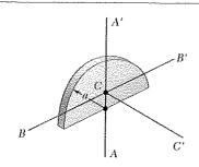
A thin semicircular plate has a radius a and a mass m. Determine the mass moment of inertia of the plate with respect to (a) the centroidal axis BB', (b) the centroidal axis CC' that is perpendicular to the plate.
