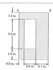
Determine the moments of inertia  $\overline{I}_x$  and  $\overline{I}_y$  of the area shown with respect to centroidal axes respectively parallel and perpendicular to side AB.
