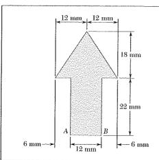
Determine the moments of inertia  $\overline{I}_x$  and  $\overline{I}_y$  of the area shown with respect to centroidal axes respectively parallel and perpendicular to side AB.
