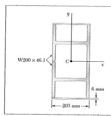
To form a reinforced box section, two rolled W sections and two plates are welded together. Determine the moments of inertia and the radii of gyration of the combined section with respect to the centroidal axes shown.
