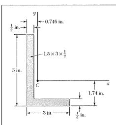
For the L5  $\times$  3  $\times$   $\frac{1}{2}$ -in. angle cross section shown, use Mohr's circle to determine (a) the moments of inertia and the product of inertia with respect to new centroidal axes obtained by rotating the x and y axes 30° clockwise, (b) the orientation of the principal axes through the centroid and the corresponding values of the moments of inertia.
